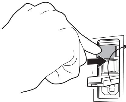
**Figure 4-33 Install the Fuse Holder**
