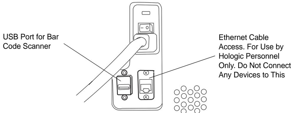
**Figure 2-8 USB Port for Bar Code Scanner**
