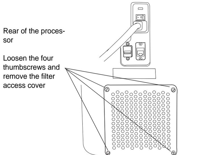
**Figure 4-9 Remove the Filter Access Cover**
