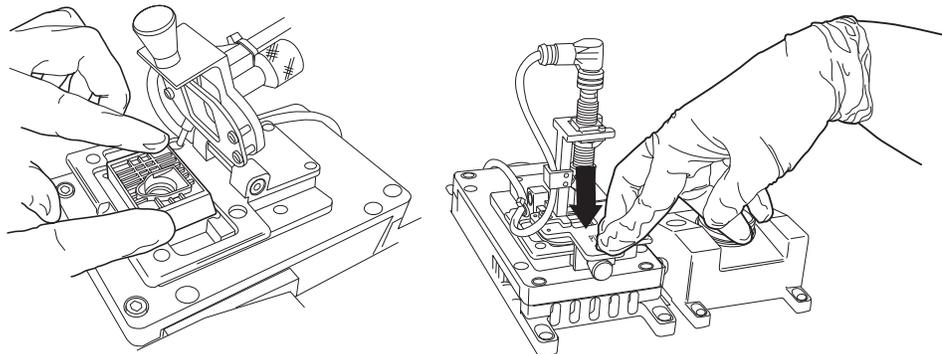
**Figure 3-8 Load the Cassette/Filter Assembly into the Cassette Holder**
