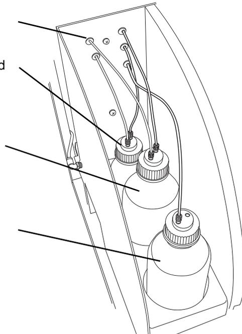
**Figure 2-5 Reagent Bottles and Manifold Connectors**
