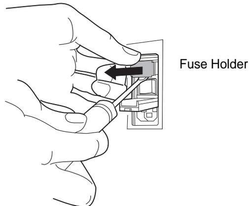
**Figure 4-31 Remove the Fuse Holder**
