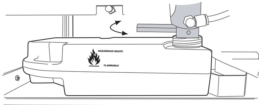
**Figure 4-6 Remove/Replace Waste Collection Tank**
