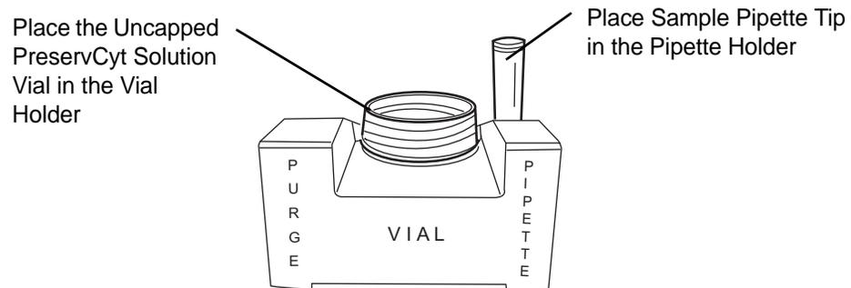
**Figure 3-7 Load Sample Vial and Sample Pipette Tip**
