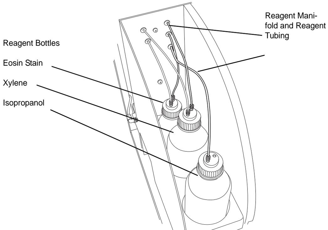
**Figure 1-4 Reagent Compartment**
