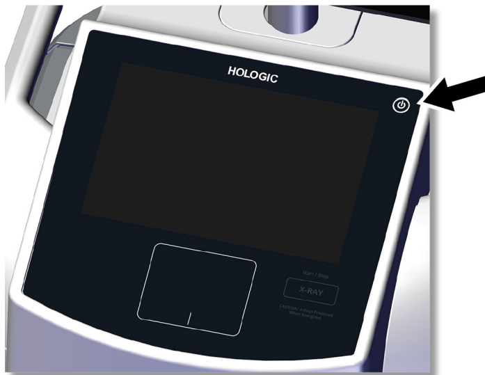
Figure 8: Computer Power Switch
